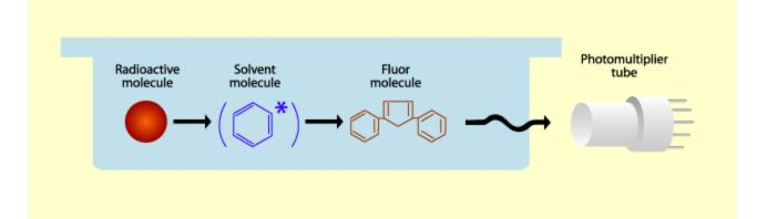
The beta decay electron emitted by the radioactive isotope in the sample excites the solvent molecule which in turn transfers the energy to the solute (called a fluor as it emits light). The fluor emits a photon of light that is detected by the photomultiplier tube and converted into an electric signal and detected by the apparatus.
