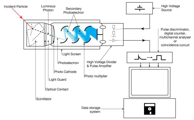
Apparatus with a scintillating crystal, photomultiplier, and data acquisition components.
