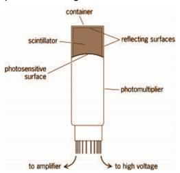
A scintillation counter is used to detect gamma rays and a presence of a particle. It can also measure the radiation in the scintillating medium, the energy loss or the energy gain. The medium can either be gaseous, liquid or a solid. The scintillator counter is generally comprised of the transparent crystalline material such as glasses, liquids or plastics. One sector of the scintillators is placed (optical contact )with the pin code.
