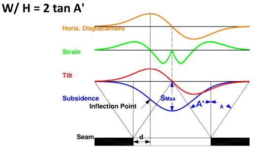
**SuperCritical Panel: A SuperCritical** panel is so wide in relation to the depth (H) that the lines denoting the internal angle-of-draw do not cross or meet before they reach the surface. The maximum possible subsidence is obtained at all points between the surface intersections of the internal angle-of-draw lines.
