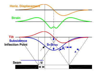
The **Maximum Possible Subsidence (Smax)** is the maximum vertical surface displacement for a panel that is wide enough that the edges do not limit the subsidence in the center of the panel (a critical or supercritical panel).
