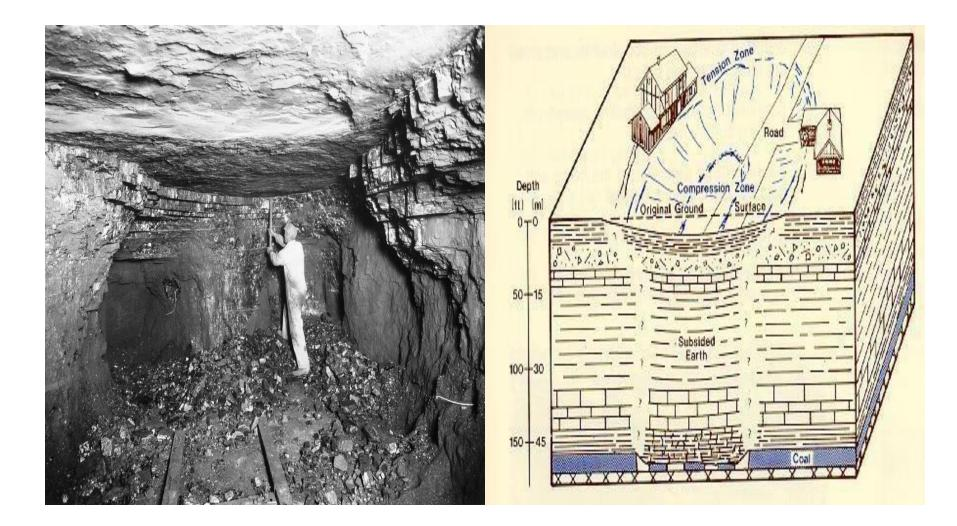
What happens when we pull pillars or extract a longwall panel? The ground moves in to fill the opening created by the full extraction. The overburden loses the sub-adjacent support and falls into the void created by removing the coal or seam material. This is known as **Subsidence**. **Overburden Zones -** The ground movement occurs in 3 or 4 zones which can be differentiated from each other by severity of strata disturbance.
