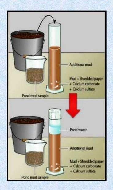
The added organic material initially triggers microbial activity that depletes the oxygen in the mud.
