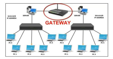
A gateway operates on all the layers of the OSI model, so it can be used as a one-stop solution for all kinds of network device connectivities.
