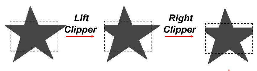
At each step, a new sequence of output vertices is generated and passed to the next window boundary clipper.
