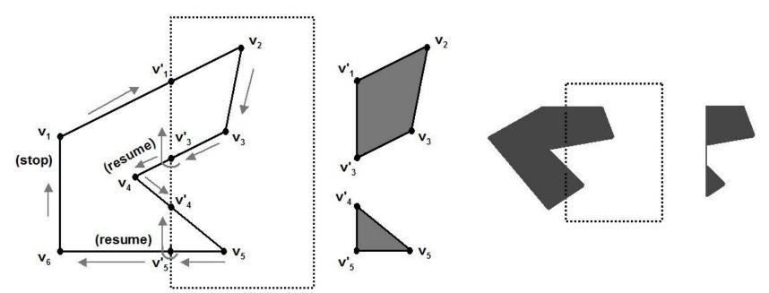
Clipped Polygon using Weiler-Atherton Polygon Clipping without connected component problem Clipped Polygon using sutherland hogman algorithm with connected component problem
