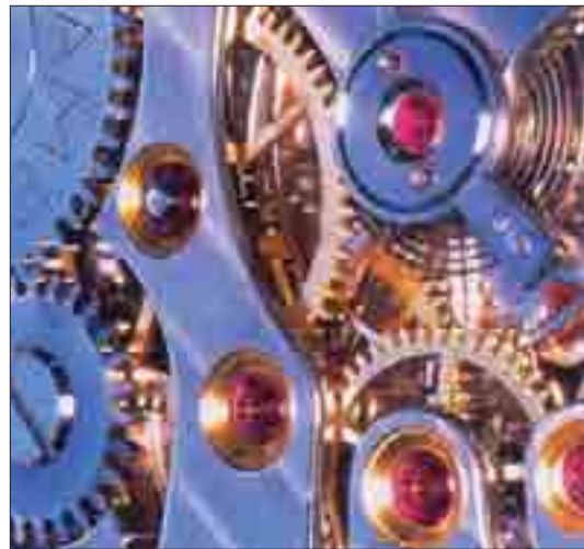
Gear trains inside a mechanical watch
