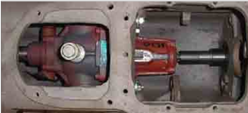
Hydrostatic transmission inside a tractor engine
