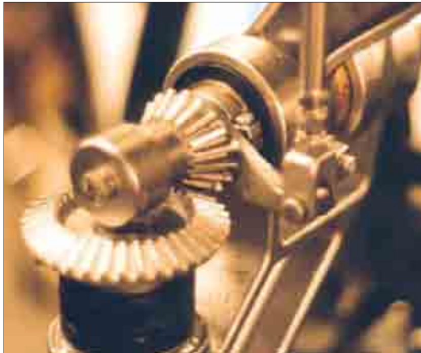
Fig. 30.1. Pitch surface for bevel gears.
