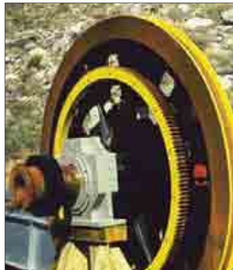
Wheel that winds the metal rope.
