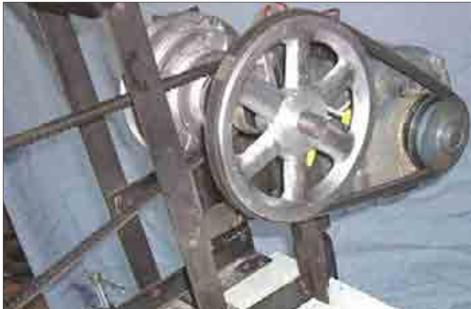
Belt drive on a lathe
