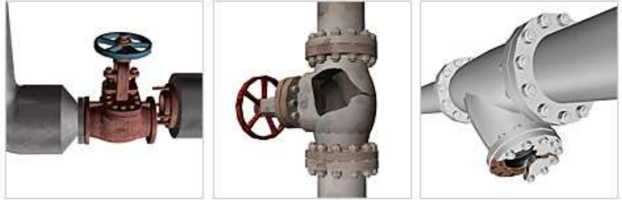
Example of piping damaged by water hammer
