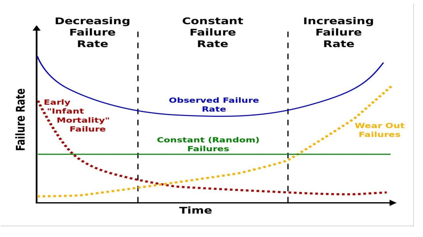
The **bathtub curve** is widely used in reliability engineering. The name is derived from the cross-sectional shape of a bath tub- steep sides and a flat bottom.
