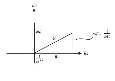
We note that the reactance may be positive or negative according to the relative values of  $\omega L$  and  $1/\omega C$ . Indeed at a frequency  $\omega = \sqrt{LC}$  we see that X=0 and that the impedance is purely resistive. We will return to this point later.
