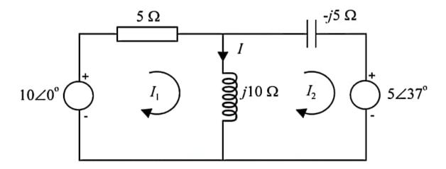
The reactances have been calculated and marked on the diagram. The left hand voltage source has been chosen as reference and provides 10V rms. The right hand source produces 5V rms but at a phase angle of  $37^\circ$  with respect to the 10V source. If we introduce *phasor loop currents I*<sub>1</sub> and *I*<sub>2</sub> as shown then we may write KVL loop equations as
