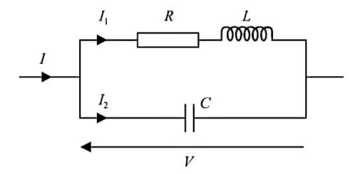
We could obtain the relationship between *I* and *V* by using the equivalent impedance derived earlier. However we will use a phasor diagram to show the various currents and voltages which appear across the various components. Since the voltage, *V*, is the same across each arm it is sensible to choose this as the reference phasor.
