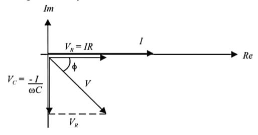
from which it is clear that the voltage lags the current by an angle  $\phi$ . The angle  $\phi$  may be obtained from the diagram as  $\phi$ =tan  $^1$ (1/ $\omega$ CR).
