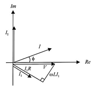
where  $\phi$  denotes the phase angle between V and I. In the diagram above I leads V by  $\phi.$
