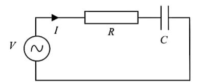
Since the current, I, flows through both elements it is sensible to choose this as the *reference* phasor. Having made this choice the voltage drop across the resistor,  $V_R = IR$ , whereas that across the capacitor,
