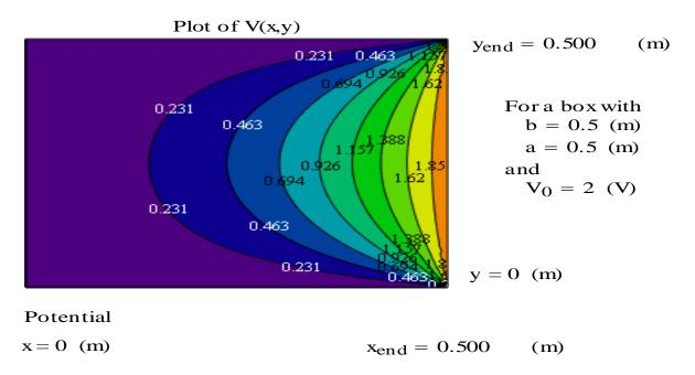
We can observe in this plot that the potential is a complicated function of x and y. (The plot below may help in visualizing the variation of V throughout the interior of this bose potential is symmetric about the plane y = a/2 which we would expect since the box boundary conditions are both symmetric about this same plane.
