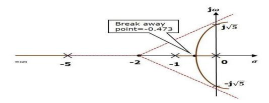
In this way, you can draw the root locus diagram of any control system and observe the movement of poles of the closed loop transfer function. From the root locus diagrams, we can know the range of K values for different types of damping.
