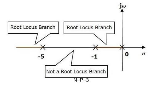
The three poles are located are shown in the above figure. The line segment between s=-1, and s=0 is one branch of root locus on real axis. And the other branch of the root locus on the real axis is the line segment to the left of s=-5.
