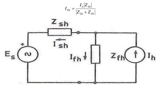
The harmonic voltage at the converter bus is
