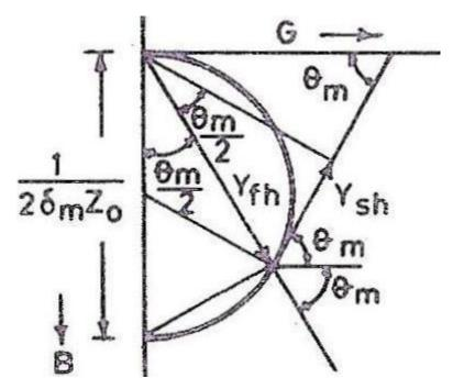
The optimum value of Q can be obtained from game-theoretic analysis. If one selects  $Y_{Fh}$  arbitrarily (the tip of  $Y_{Fh}$  lying along the semicircle), the network can select  $Y_{Sh}$  such that the vector  $Y_h$  is perpendicular to the vector  $Y_{Sh}$  and ensure  $Y_h$  is minimum. To maximize the minimum magnitude of  $Y_h$ , it is necessary to have  $Y_{Sh}$  tangential to the circle. Thus, we select  $Y_{Fh}$  to maximize  $Y_h$  when the network tries to minimize it.
