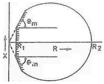
The value of  $Y_h$  is reduced if the detuning parameter  $\delta$  is maximum =  $\delta_m$ . For a specified value  $\delta_m$  and  $X_0$ , the locus of the filter impedance as Q is varied is a semicircle in the 4<sup>th</sup> quadrant of the G-B plane as shown below.
