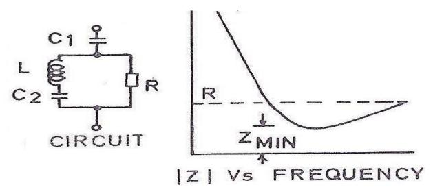
A converter system with 12 pulse converters has Double Tuned (or two Single Tuned) Filter banks to filter out 11<sup>th</sup> and 13<sup>th</sup> harmonics and a High Pass Filter bank to filter the rest of harmonics. Sometimes a third harmonic filter may be used to filter the non-characteristic harmonics of the 3<sup>rd</sup> order particularly with weak AC systems where some voltage unbalance is expected.
