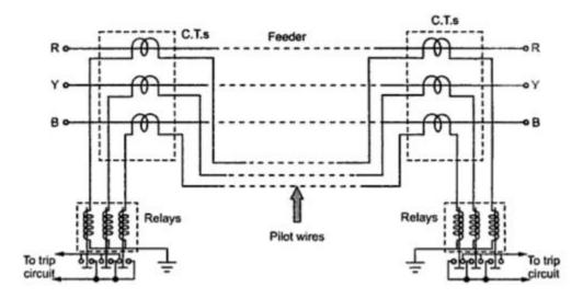
Under normal condition, current entering the line at one end is equal to current leaving from the other end. Therefore, equal and opposite voltages are induced in the secondaries of C.T.s. at the two ends resulting in no current flow, through the relay.
