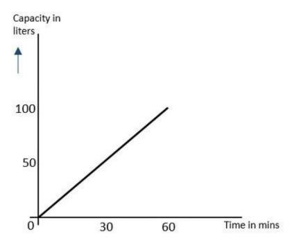
As the result shown in this image varies (increases) according to time, this time varying quantity can be understood as Analog quantity. The signal which represents this condition with an inclined line in the figure, is an **Analog Signal**. The communication based on analog signals and analog values is called as **Analog Communication**.
