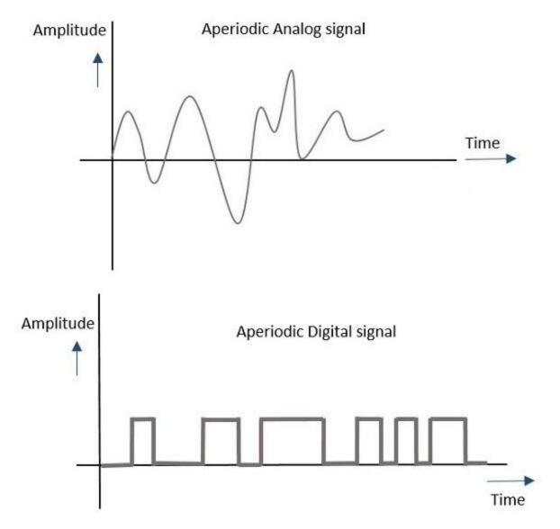
In general, the signals which are used in communication systems are analog in nature, which are transmitted in analog or converted to digital and then transmitted, depending upon the requirement.
