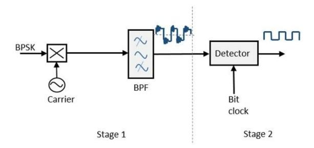
By recovering the band-limited message signal, with the help of the mixer circuit and the band pass filter, the first stage of demodulation gets completed. The base band signal which is band limited is obtained and this signal is used to regenerate the binary message bit stream.
