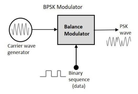
The modulation of BPSK is done using a balance modulator, which multiplies the two signals applied at the input. For a zero binary input, the phase will be **0**° and for a high input, the phase reversal is of **180**°.
