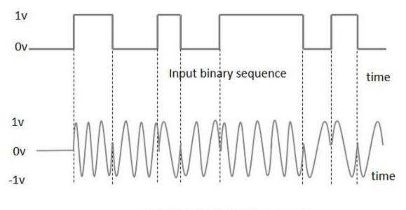
BPSK Modulated output wave
