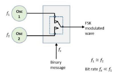
The two oscillators, producing a higher and a lower frequency signals, are connected to a switch along with an internal clock. To avoid the abrupt phase discontinuities of the output waveform during the transmission of the message, a clock is applied to both the oscillators, internally. The binary input sequence is applied to the transmitter so as to choose the frequencies according to the binary input.
