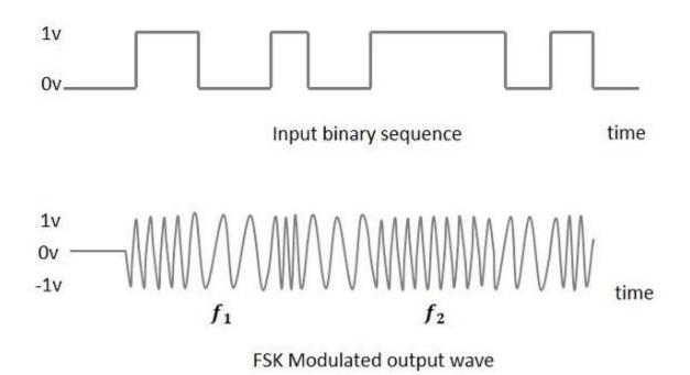
To find the process of obtaining this FSK modulated wave, let us know about the working of a FSK modulator.
