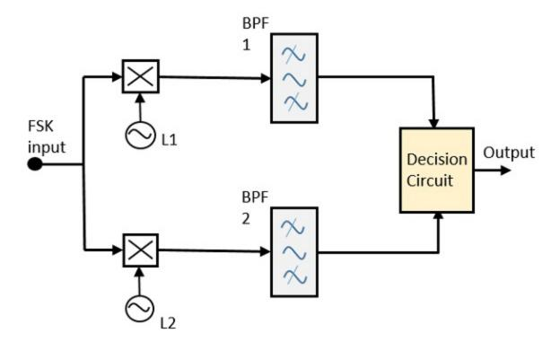
The FSK signal input is given to the two mixers with local oscillator circuits. These two are connected to two band pass filters. These combinations act as demodulators and the decision circuit chooses which output is more likely and selects it from any one of the detectors. The two signals have a minimum frequency separation.
