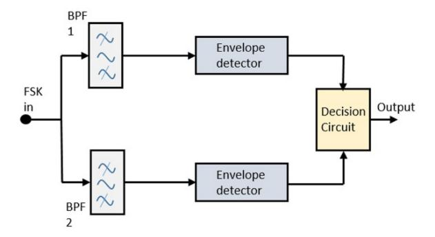
The FSK signal is passed through the two Band Pass Filters BPFsBPFs, tuned to **Space** and **Mark** frequencies. The output from these two BPFs look like ASK signal, which is given to the envelope detector. The signal in each envelope detector is modulated asynchronously.
