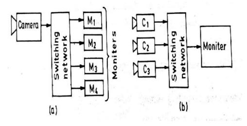
In diagram (a) a single camera(C) is connected to many monitors (M) through switching network (SN).in this we can see a single program in monitors at many places.
