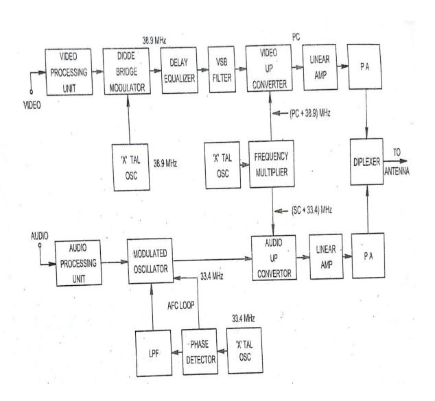
In this video modulation is done at IF frequency of 38.9 MHZ and sound modulation is done at IF frequency of 33.4 MHZ. Both video and sound IF UP converted after modulation. A VSB filter is also included at lower IF power level. After up conversion they are given to lines, amplifier for power amplification and then it is connected to the diplexer unit.
