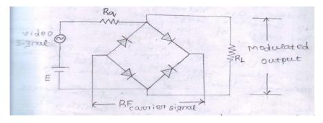
A bridge diode modulator or a diode balanced modulator is used for LLM.
