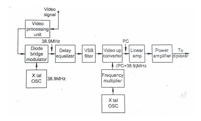
Visual exciter deals with circuits related to video signals. It consists of video processing unit, video modulator, VSB filter, Delay equalizer, Frequency up converter, Linear and power amplifier.
