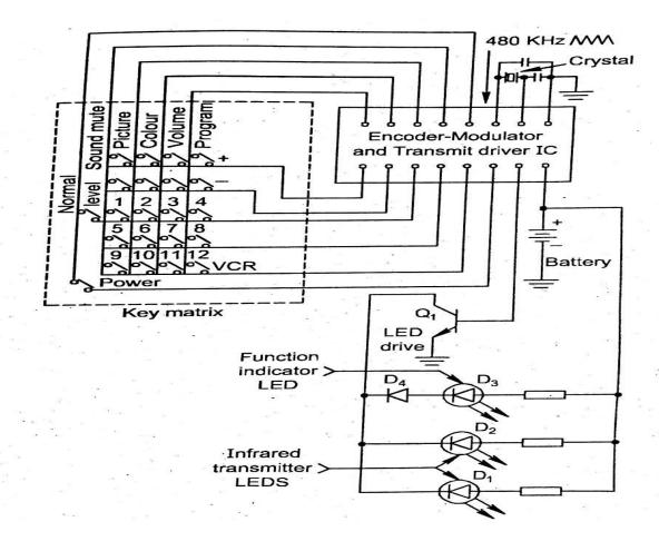
To achieve all the necessary basic function 24 different commands are needed. So 24 different pulse patterns are generated. The modulator IC (encoder) performs the main function.
