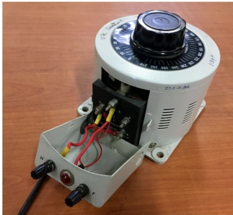
Figure 2: A 2.3 kVA, 10A single phase variac
