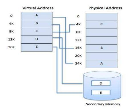
Virtual memory is commonly implemented by demand paging. It can also be implemented in a segmentation system. Demand segmentation can also be used to provide virtual memory.
