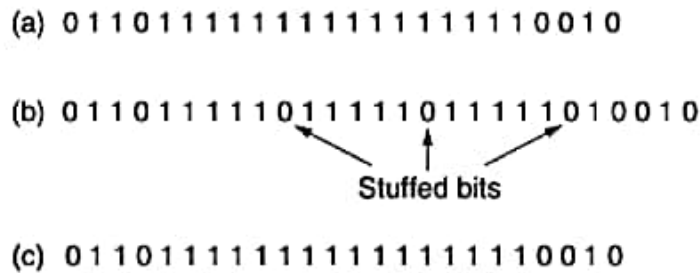
Figure 3-5. Bit stuffing. (a) The original data. (b) The data as they appear on the line. (c) The data as they are stored in the receiver's memory after destuffing.
