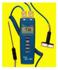
These are thermocouples which measures for example flue gas, hot air, hot water temperatures by insertion of probe into the stream. For surface temperature, a leaf type probe is used with the same instrument.
