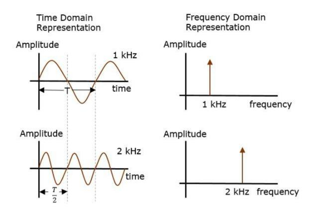
Time domain analysis, gives the signal behavior over a certain time period. In the frequency domain, the signal is analyzed as a mathematical function with respect to the frequency.
