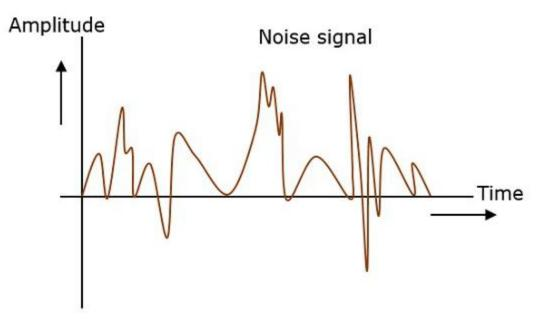
Hence, it is understood that noise is some signal which has no pattern and no constant frequency or amplitude. It is quite random and unpredictable. Measures are usually taken to reduce it, though it can't be completely eliminated.
