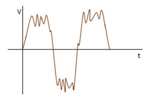
The frequency of the original signal may be 1 kHz, but the noise of certain frequency, which corrupts this signal is unknown. However, when the same signal is represented in the frequency domain, using a spectrum analyzer, it is plotted as shown in the following figure.
