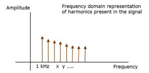
Here, we can observe few harmonics, which represent the noise introduced into the original signal. Hence, the signal representation helps in analyzing the signals.
