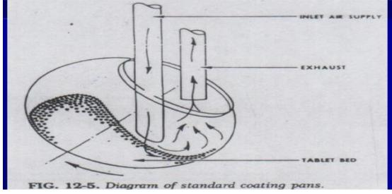
**Process:** The core material is sieved to remove the dust particles and then added to the coating pan. The coating material is then added through coating solution inlet and moreover with the aid of spray nozzle it gets sprayed on the core material till the desired thickness is obtained. Excess solvent is removed by passing warm air.<sup>[87,88.]</sup>
