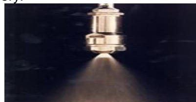
Fig. 2: Spray drying technology: nozzle atomizer in a spray dryer 19
